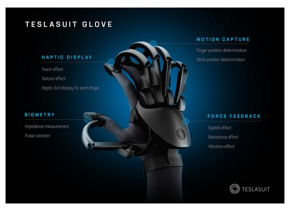
${\it TESLASUIT\ Glove, an\ exoskeleton\ force\ feedback\ glove\ used\ in\ conjunction\ with\ the\ {\it TESLASUIT\ }}$
